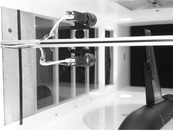
Fig. 5 PIV experiment setup.
